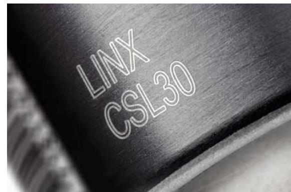
Laser coding of coated aerosols
