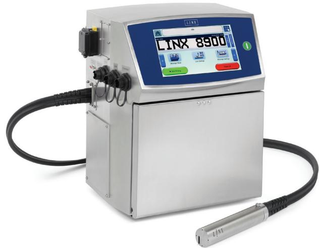
A particular benefit of the Linx 8900 for Fourpure is its ability to deliver excellent quality codes from the moment it starts up, even if run intermittently. The Linx 8900 features Linx's proven autoflush system which thoroughly cleans the printhead every time it is shut down for a fast and clean startup when next required.
