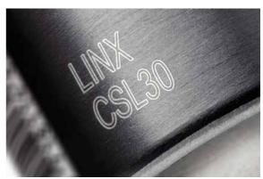
Laser coding of coated aerosols
