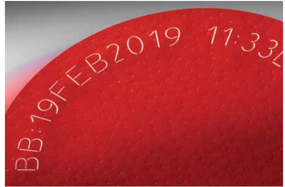
Laser marking onto plastic coated dessert lid
