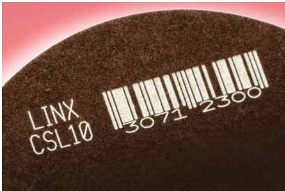
Laser marking onto painted card packaging
