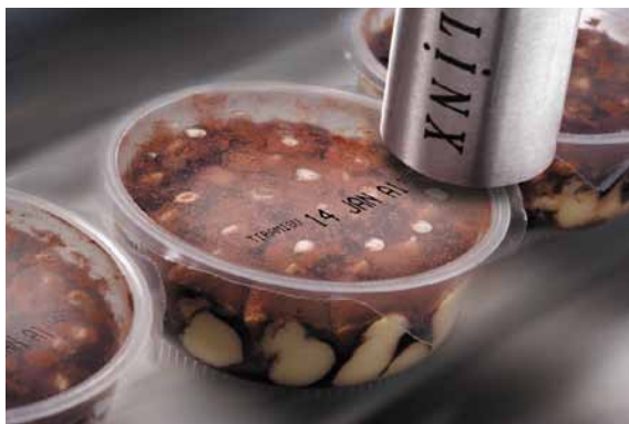
CIJ ink penetrating through condensation
