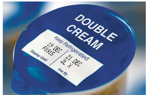
CIJ printing onto plastic
