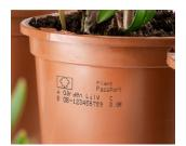
Linx Dutch distributor, De Koningh BV, is working with plant producers in the Netherlands to find the perfect solution to meet the new EU regulations for plant passports. Customers are choosing to install Linx 8920 and 8940 small character continuous ink jet printers onto their potting lines to apply the new format plant passports onto every plant pot, box or tray as they move along the potting line.
