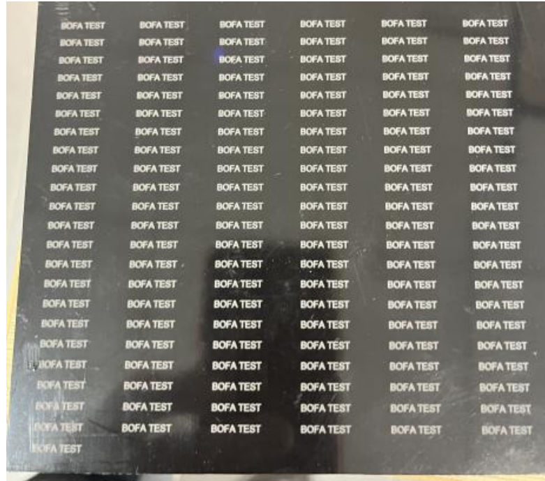
Figure 11 achieved laser mark HDPE
