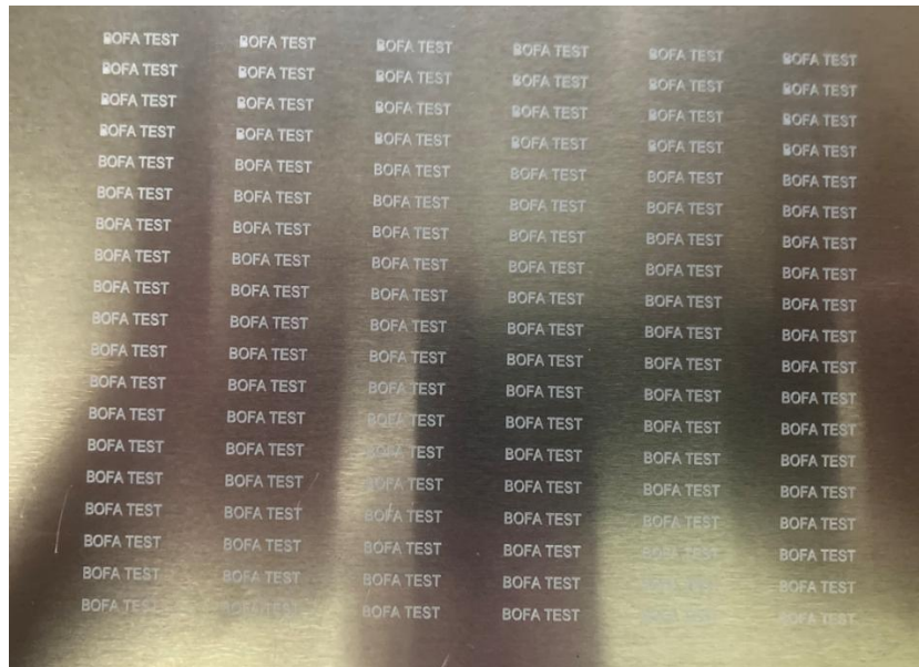
Figure 12 achieved laser mark aluminium
